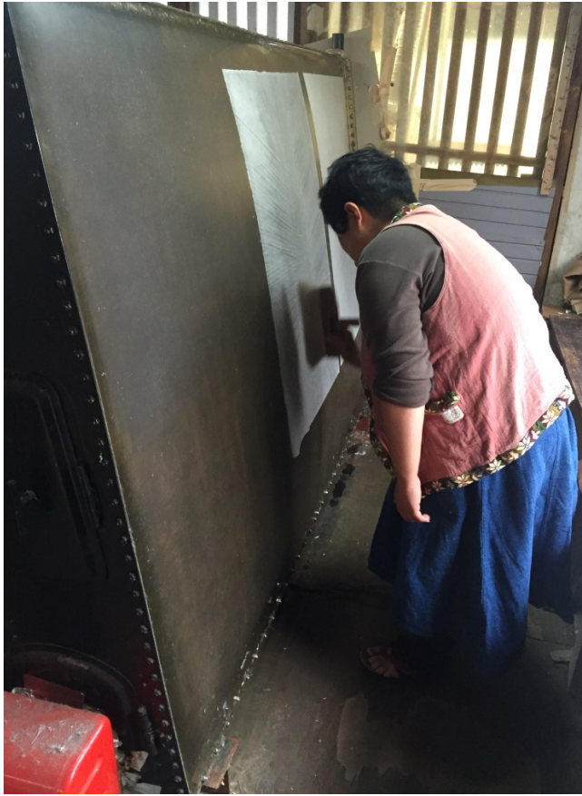
Figure 41 - Mino. Mrs. Senda applying a freshly-made sheet of paper to the electric drying machine.
