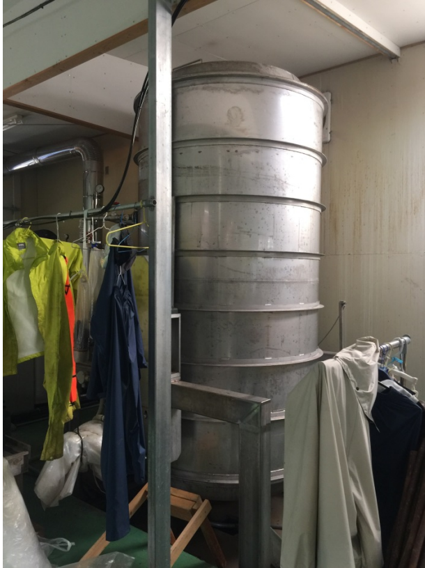
Figure 50 - Tosa. The custom-built steaming drum.
