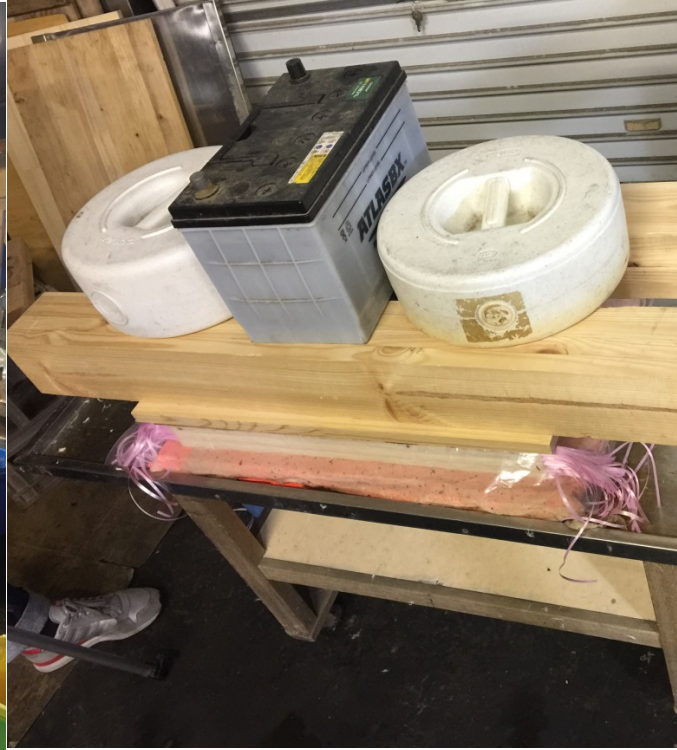
Figure 76 - Shiroishi. Mr.A uses old car batteries instead of a paper press to remove water.
