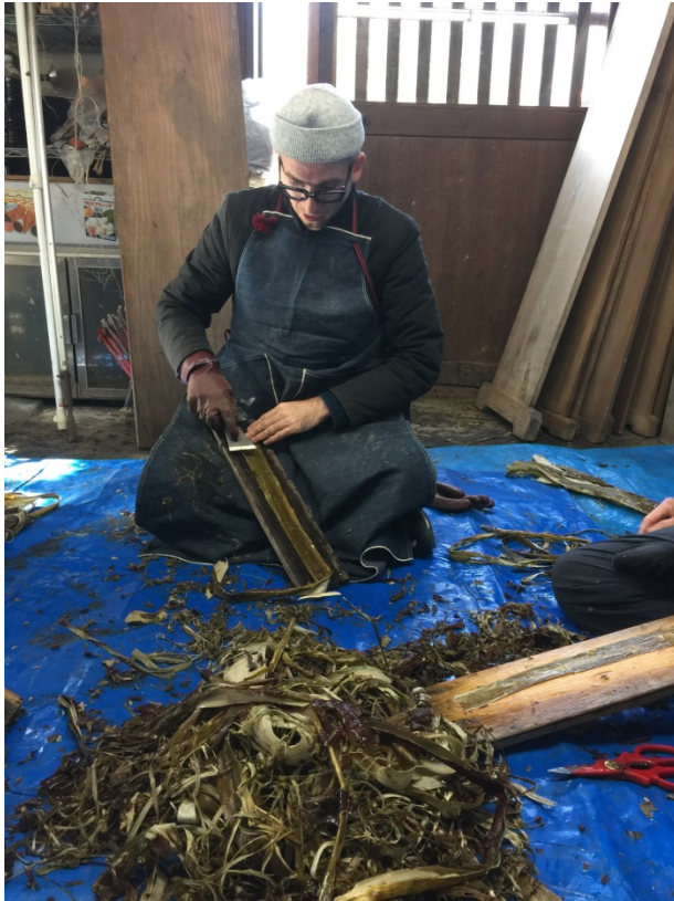
Figure 34 - Ogawamachi. Removing the black bark with a putty knife.
