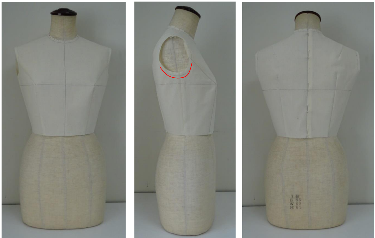
Fig.2-16 Toile check of three-dimensional pattern by peeling the surface of the virtual body (Upper body)
