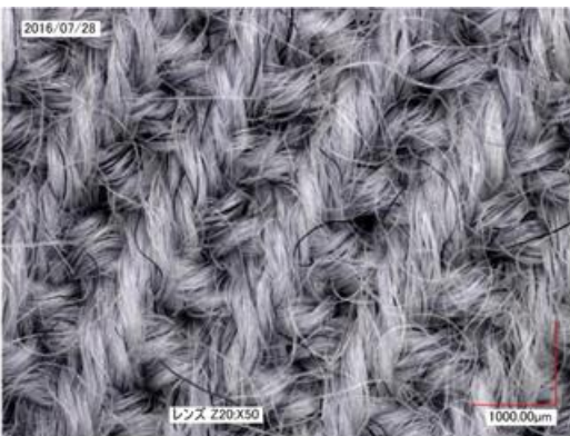
Fig.4-13 Microscope image and organization chart of Kersey 3×3
