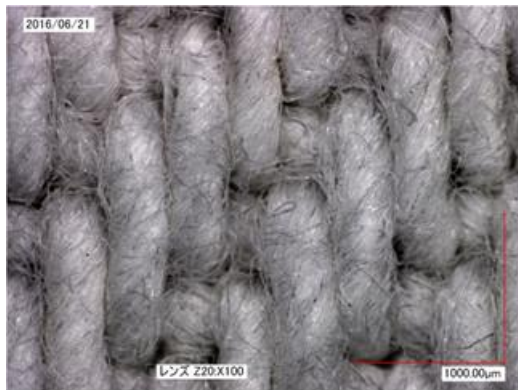
Fig.4-8 Microscope image and organization chart of Denim
