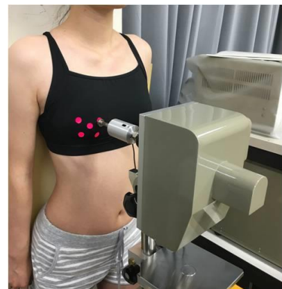
Fig.2.10 Posture of breast compression measuring
