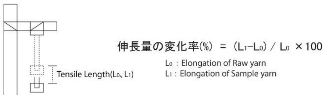
Fig. 5.5 The method for Change of stretch length
