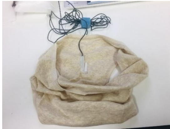
Fig. 5-6 A sensor wrapped in a moisture permeable waterproof cloth
