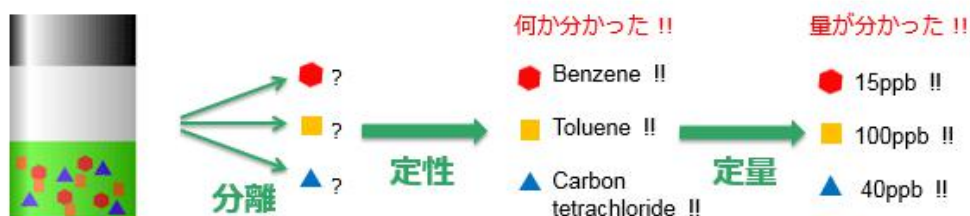
Fig.4-6 Qualitative analysis and quantitative analysis mode diagram 24)
