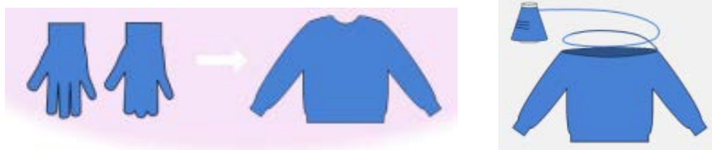
Fig. 2.4 The evolution from glove to WHOLEGARMENT® 3)5)
