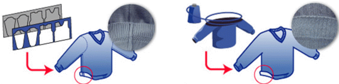
Fig. 2.6 Comparison of legacy knitwear (Left) and seamless knitwear (Right) 4)
