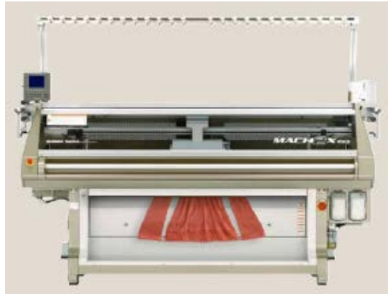
Fig. 2.3 Seamless Machine (1995~) WHOLEGARMENT® 4)
