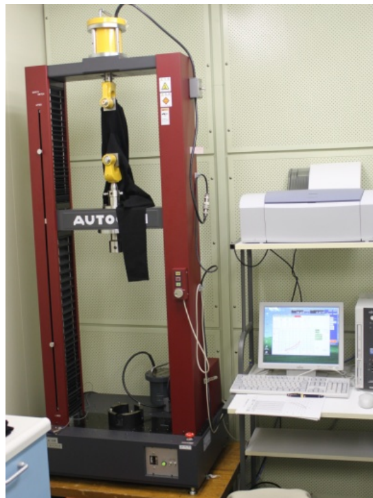
Fig. 4.1 Tensile testing machine (Auto COM/AC-100) (in the Constant temperature and humidity room)
