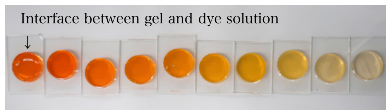
Fig. 4.3 Agar gel cut into rings at 5mm intervals for measurement
