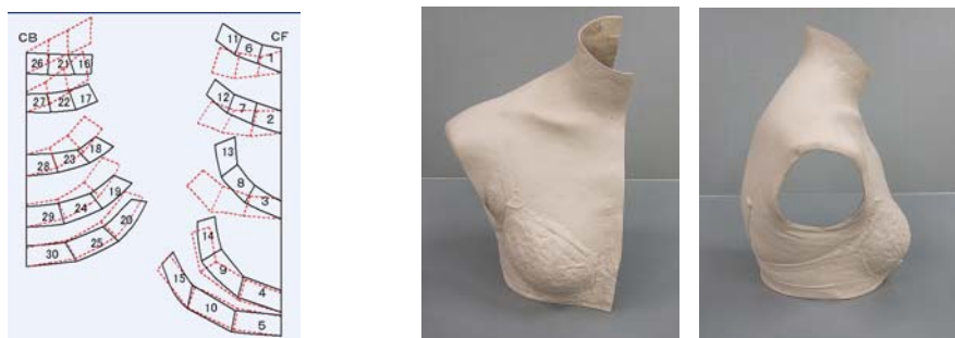
Fig.3 Neck plaster measurement procedure (left: Unfolding of washi paper, right: Plastic specimen)
