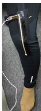
Fig.11 High molecular polymer sensor for measuring knee bend (left) and its implementation on a stretchable pants (right) 膝関節計測用高分子ポリマーセンサー試作(左)と膝部への実装の様子(右)
