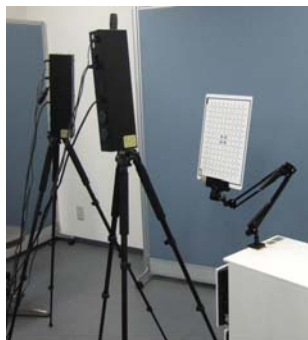
Fig.1 CARTESIA 3D Handy Scanner
